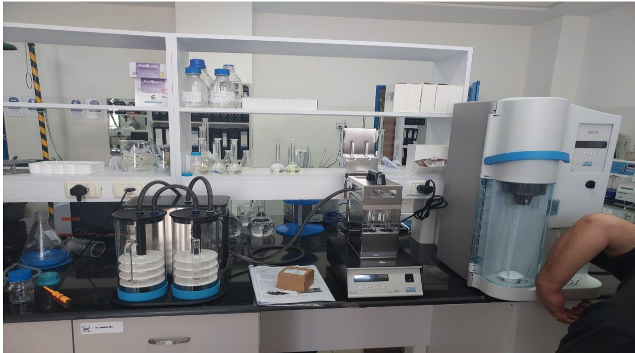
Figure (1): Digestion Unit. This system is used to analyze food and agrifood ingredients.
