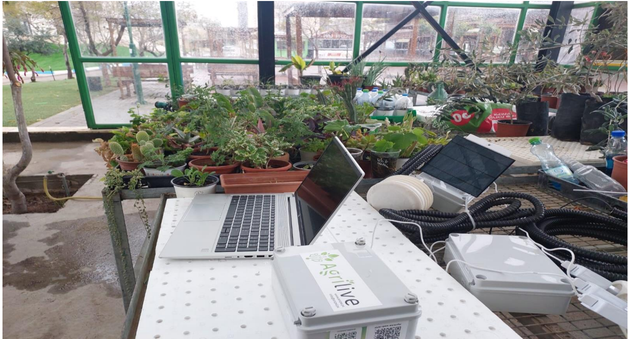
Figure (3): Agri-live system for the monitoring of temperature, humidity, ph and other crop parameters
