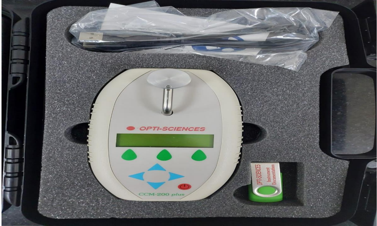
Figure (5): Chlorophyll meter for the measurements of crop health.
