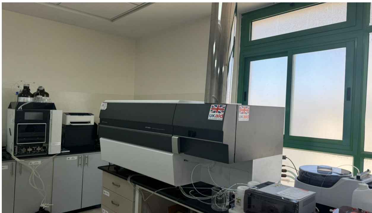
Figure (11): HPLC and ICP for agrifood chemical analysis
