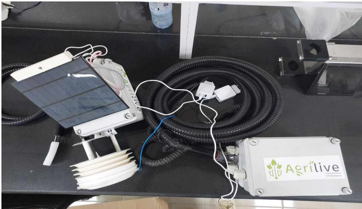
Figure (4): Agri-live system for the monitoring of temperature, humidity, ph and other crop parameters
