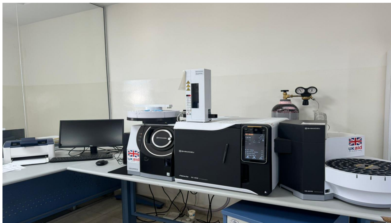
Figure (12): GC-MS for agrifood chemical analysis
